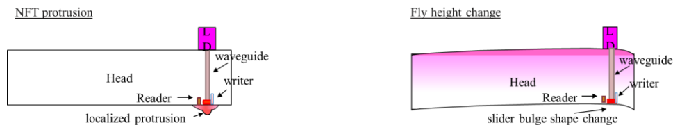
Figure 1 Laser induced protrusion in HAMR (a) localized NFT protrusion (b) fly height change due to slider crown and camber change.
